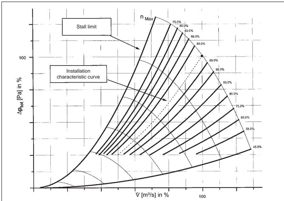
Chart 2: Characteristic curves of an axial-flow fan with rpm control based on a frequency converter
