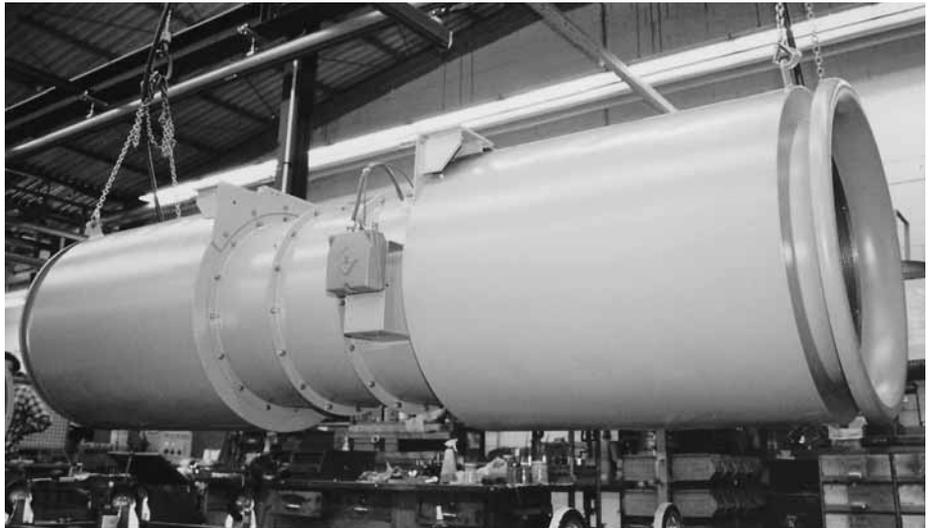
Fig. 3: Jet fan during manufacture, powder coated and with closed impeller (impeller hub sealed off against dust and corrosion)
