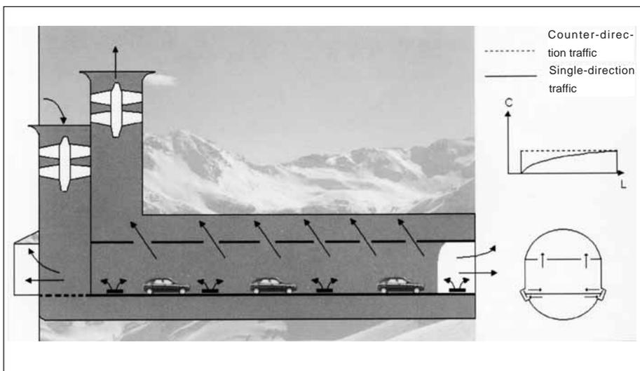
Diagram 3: Combined semi-/fully-transverse ventilation
