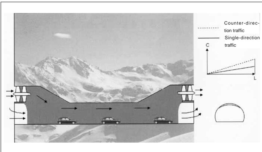
Diagram 5: Longitudinal ventilation using Saccardo nozzles
