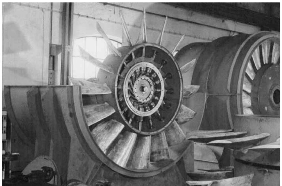
Fig. 2: Axial-flow fan with hydraulic impeller blade pitch adjustment
