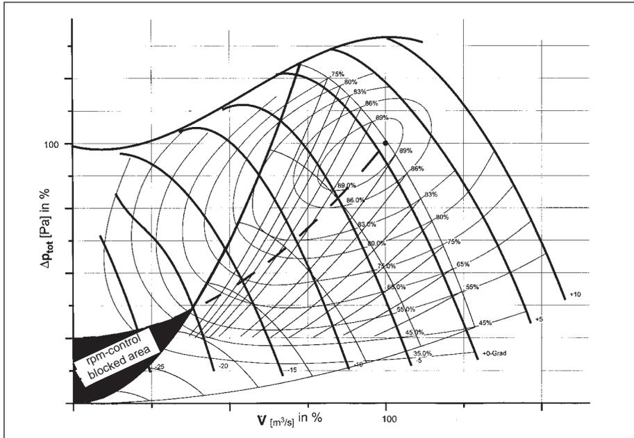
Chart 3: Characteristic curves of an axial-flow fan with hydraulic impeller blade pitch adjustment, superimposed by rpm control curves
