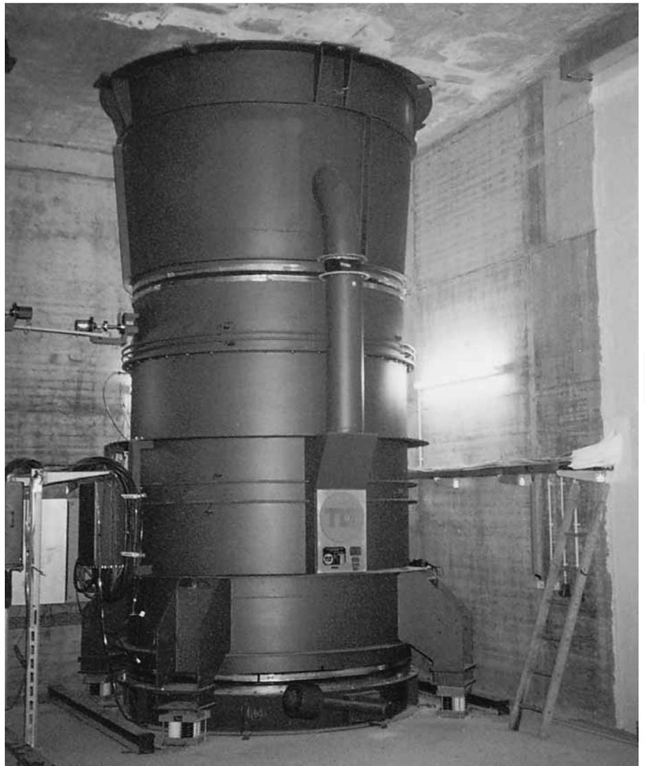
Fig. 7: Upright reversible axial-flow fan
