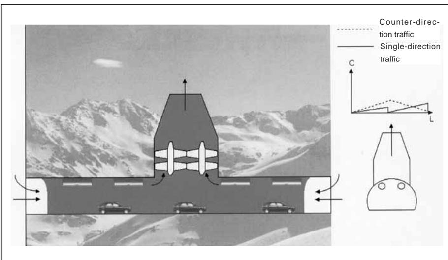
Diagram 6: Longitudinal ventilation using exhaust air fans
