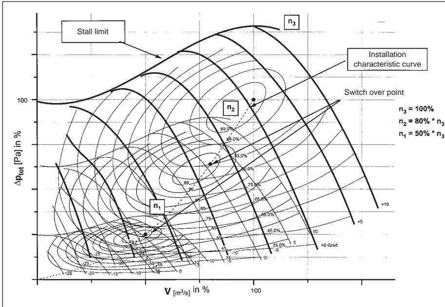
Chart 1: Characteristic curves of an axial-flow fan with hydraulic impeller blade pitch adjustment
