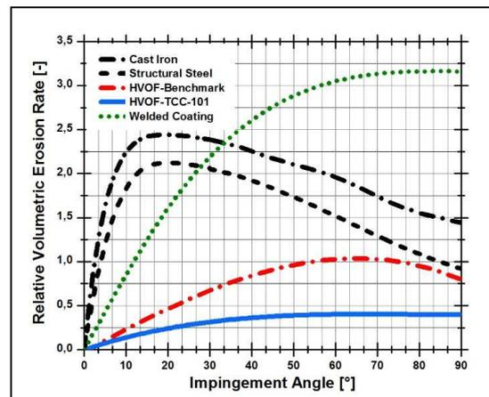
**Fig. 6:** Relative erosion rate ERR of the TLT WKB, TLT-H-101 (TCC-101), as a function of the impingement angle, as compared to standard protections and other fan materials
