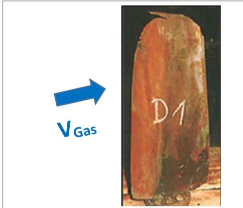
**Fig. 3:** Strong erosion of the blade of a coal fired power plant axial fan as a result of impact wear at the blade face and outlet edge
