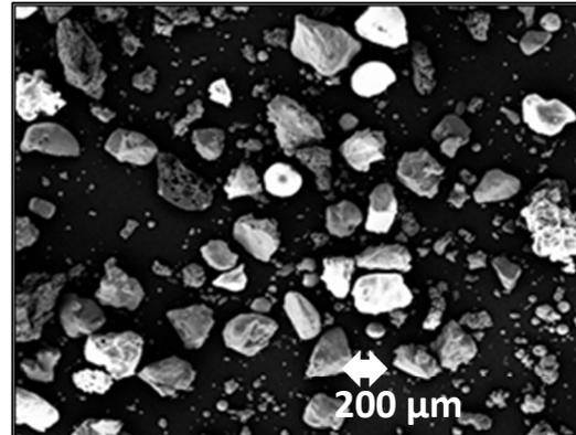
**Fig. 1:** Scanning electronic microscopy image of typical industrial abrasive ash particles
