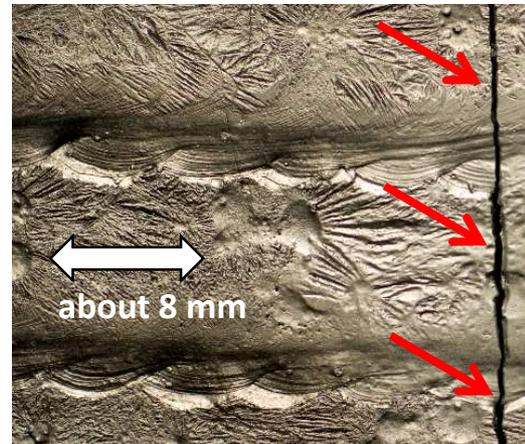
**Fig. 4:** Welded hard-facing coating with crack
