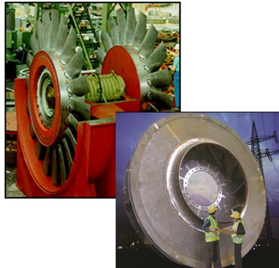
**Fig. 7:** Typical axial - and radial fan of TLT Turbo GmbH for "strong" industrial operating
