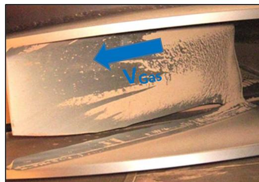
**Fig. 2:** Destruction of a centrifugal fan impeller blade close to a welding seam by particle flow erosion
