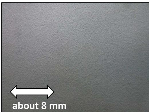
**Fig. 5:** Aerodynamically smooth, thin HVOF sprayed tungsten carbide coating on centrifugal fan impeller blade
