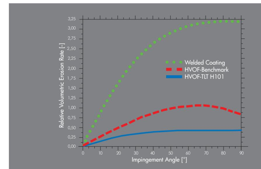
Relative wear rate due to particle impact angle
