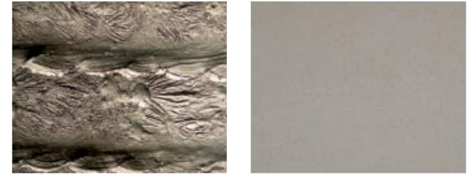
Comparison of the surface of an armored plate (left) and a HVOF-coating (right)
