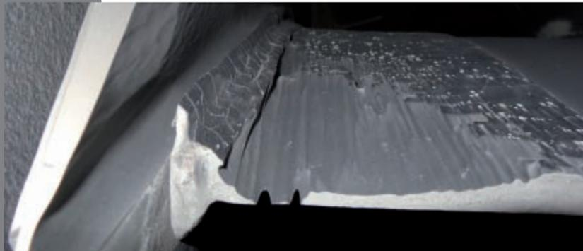
Wear in blade area at impeller outlet
