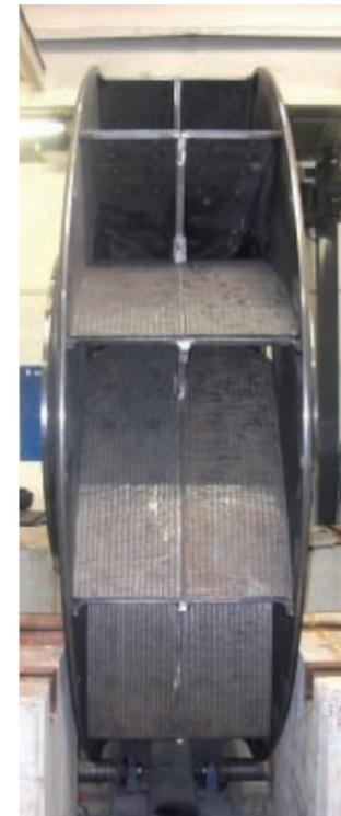
Impeller with welded composite armour plate.
