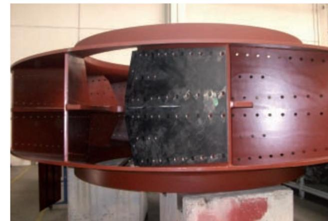
Impeller with screw-on wear protection.
